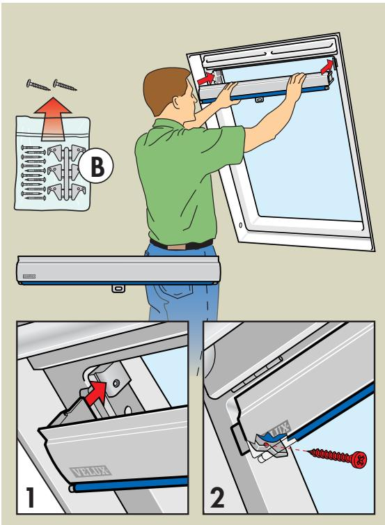
**English:** Slide blind onto brackets (1) and fix with screws supplied in bag B (2).
